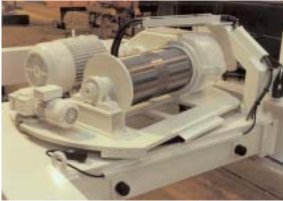
6t Special Application Rotating Hoist Channel Tunnel
